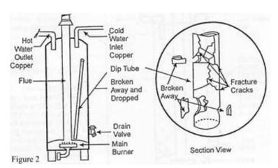
**Figure 3** shows that over time, the dip tube continues to change. Cracks and fractures from all over the dip tube surface. The turbulence created inside the tank breaks the tube into increasingly smaller pieces. The pieces are eventually flushed out of the tank through the hot water outlet. The missing dip tube also reduces the supply of hot water.
